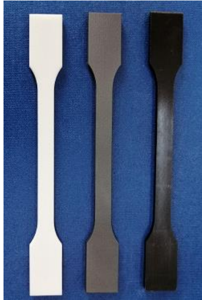
Figure 2. Tensile strength test samples (White- SLS, Grey-MJF, Black-PI)
