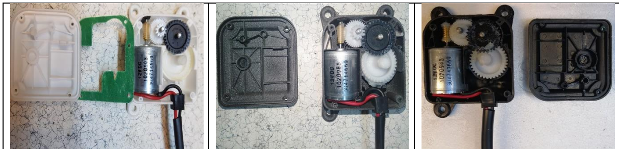
Figure 3: Flap motors with components (White- SLS, Grey-MJF, Black-PI)
